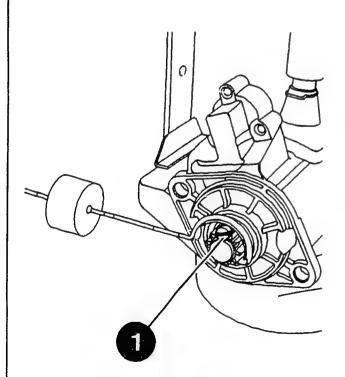
Checking armature braking torque
